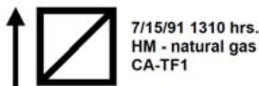
Figure 3: FEMA Structure/Hazards Evaluation Marking
