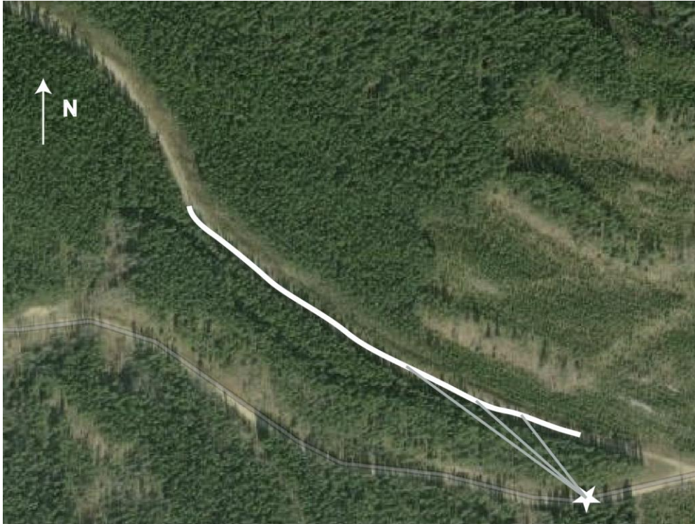
Figure 1. Satellite image captured on Oct 15, 2015 of the location of the sound detection experiments in coniferous forest. The calling location is marked by the white star. Searchers listened at points located on the white line. The three grey lines show schematic examples of straight line sound ray paths from the caller to the listeners through the forest. Copyright free satellite image courtesy of Environmental Systems Research Institute.
