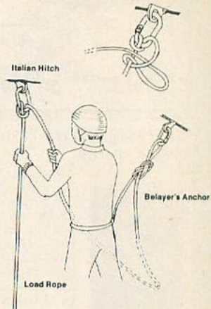
Direct belay using an Italian Hitch Belayer on separate anchor. An inset. Tying off an Italian Hitch with Half Hitch on Bight (releases under load)
