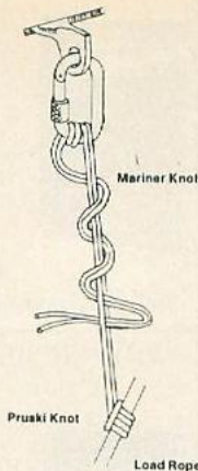
Tying off load with prusik sling fastened by a Mariner Knot (releases under load)
